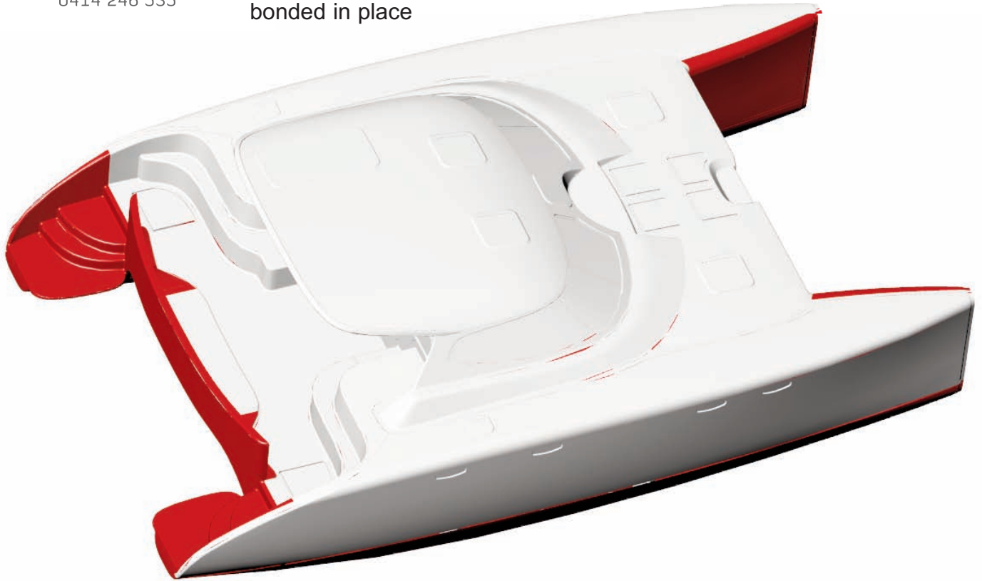
13. The final large section to go onto the boat is the cockpit seat
